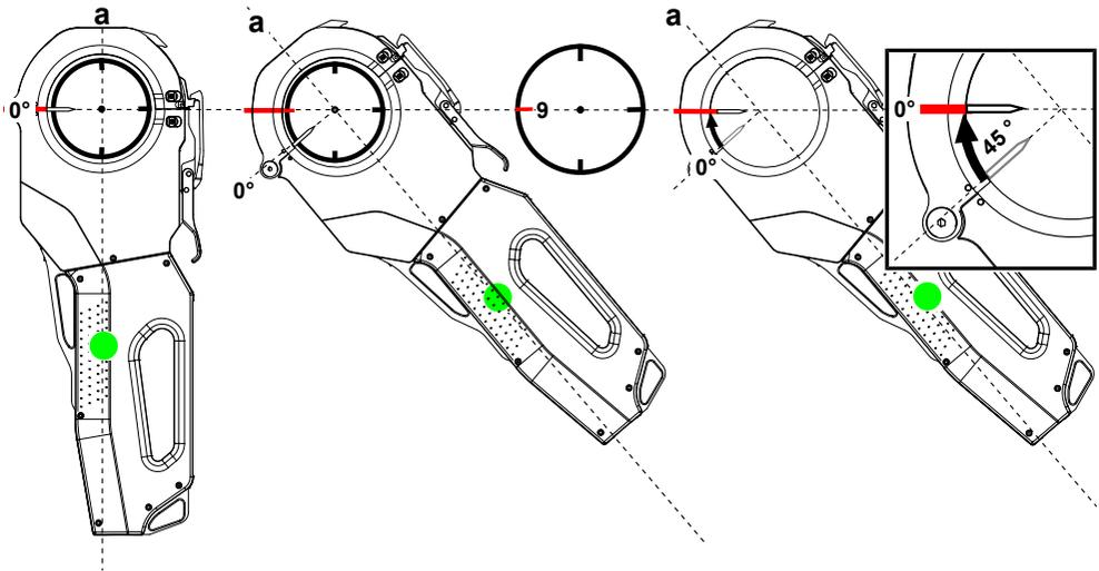
1.) The weld head is clamped on the pipe in such a way that the electrode 9 o'clock position **corresponds** to the start position in the welding procedure (0° position).
