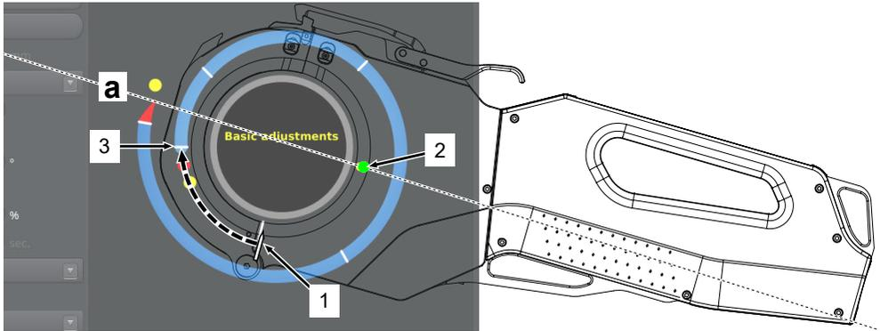
Illustration: Autopositioning of the electrode to the 9 o'clock position
