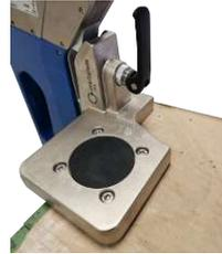
Quick clamp tilted vertically upward for stationary use.
