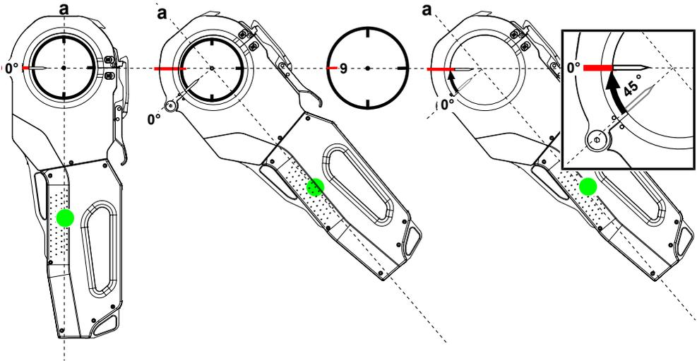
1.) The weld head is clamped on the pipe in such a way that the 9 o'clock position of the electrode **does not correspond** to the start position in the welding procedure (0° position).
