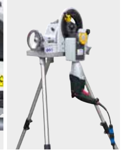
Tripod made of aluminum available optionally. Dismountable in few steps - for space-saving storage, e.g. in PS transport case
