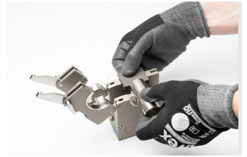
A captive pipe center gauge attached to the clamping cassette ensures the exact positioning of the pipe joint to be welded.
