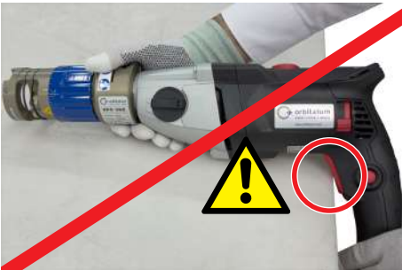
Illustration: ON/OFF button pressed against the workbench
