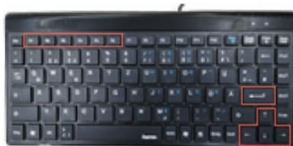
The desired control element or field can be selected with the menu cursor by means of the "up" and "down" arrow keys. The control element or field on which the menu cursor is located is highlighted in yellow. The function is activated or executed by pressing the "ENTER" key.
