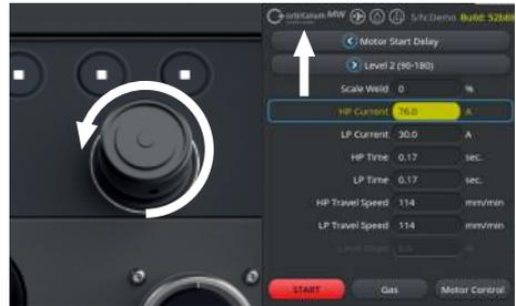
Pressing and holding the rotary control for a long time (> 2 seconds) returns you to the higher menu level.
