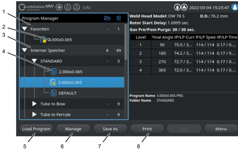
Illustration: "Manage welding procedures" softkey assignment with welding procedure marked
