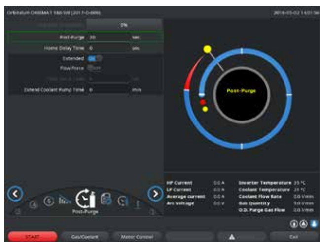
Abb. 10: Input field – Gas post purge time
