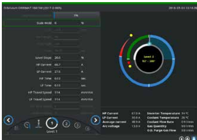
Abb. 8: Display during running welding process
