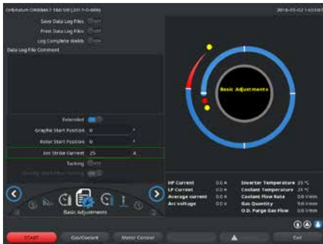
Abb. 11: Input field – Ignition current and pool formation time
