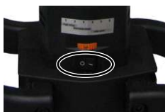
ON/OFF toggle switch on the motor
