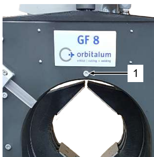
Position of the safety screw (1) on the GF 8 and GF 12 (AVM/ MVM).
