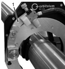
Fig.: Torch articulated arm in home position
