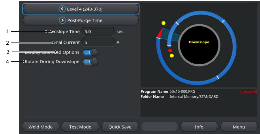
Illustration: Welding program section "Weld end"
