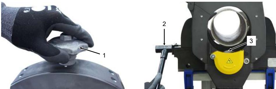
1. The slide with saw blade and supplemental bevel cutter needs to be moved all the way down by turning the star knob (1).
