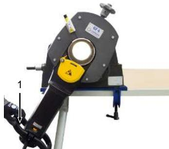
1. Adjust the pipe dimension (*see chapt. Clamping the pipe and adjusting the pipe dimension [► 50]*).
