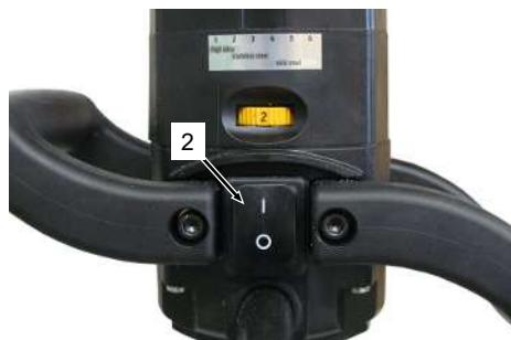
ON/OFF toggle switch on the motor
