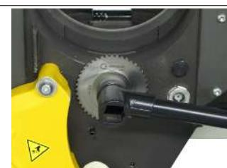
*Fixture for saw blade/bevel cutter*
