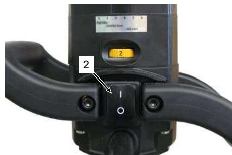
*ON/OFF toggle switch on the motor*
