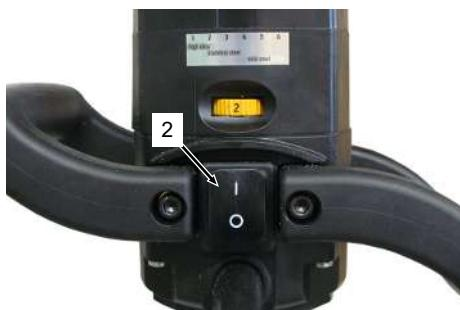
*ON/OFF toggle switch on the motor*
