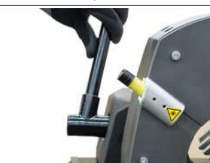
*Fixture for clamping jaws
