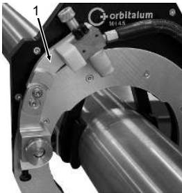
Fig.: Torch articulated arm in home position
