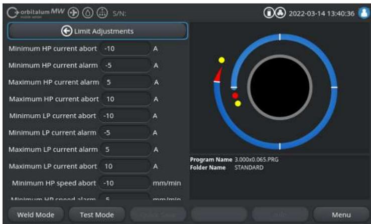
Abb.: Menu "Limit Adjustments" (Limiti parametri)
