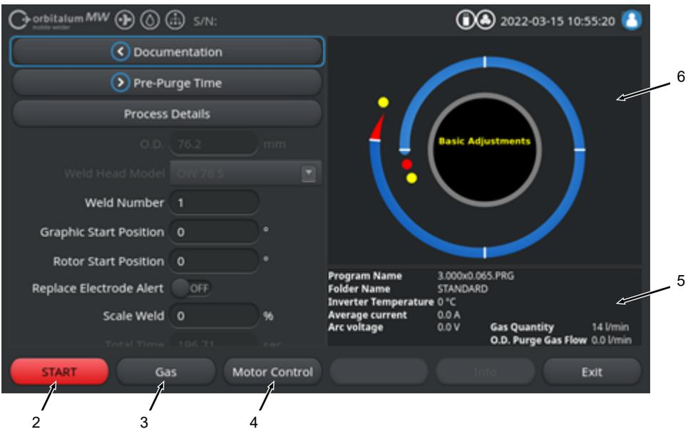
Abb.: Menu "Weld Mode" (Salda), softkey "START" rosso
