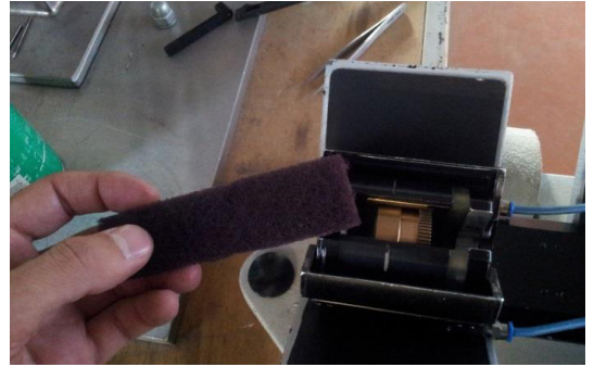
Fig. 5 Cleaning inside gear with scotch brite
