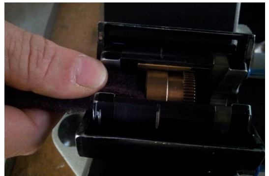
Fig. 6 Cleaning inside gear with scotch brite
