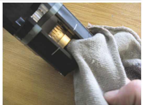
Fig. 10 Wipe current/cooling contact surface with a cloth
