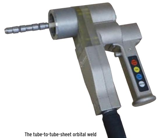
The tube-to-tube-sheet orbital weld head TX 38P:
